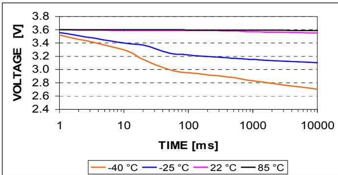
Voltage curves for HLC1550A at Li/SO<sub>2</sub>Cl<sub>2</sub> potential (3.90 V), 750 mA
