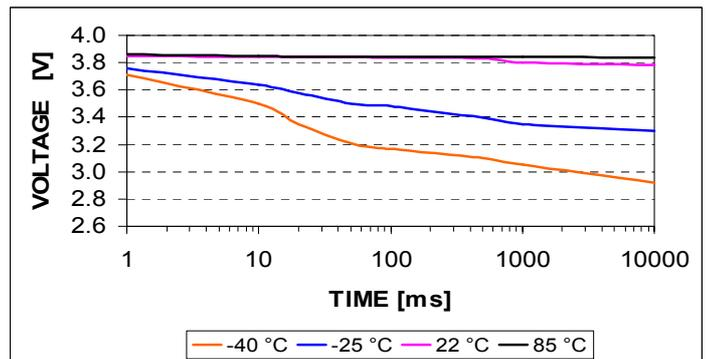
Voltage curves for HLC1550A at Li/SOCl<sub>2</sub> potential (3.67 V), 1200 mA
