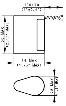
Note: For best performance battery should be mounted in the application in upright or horizontal position.
