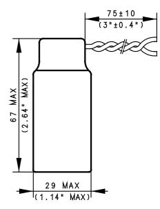
Note: For best performance battery should be mounted in the application in upright or horizontal position.
